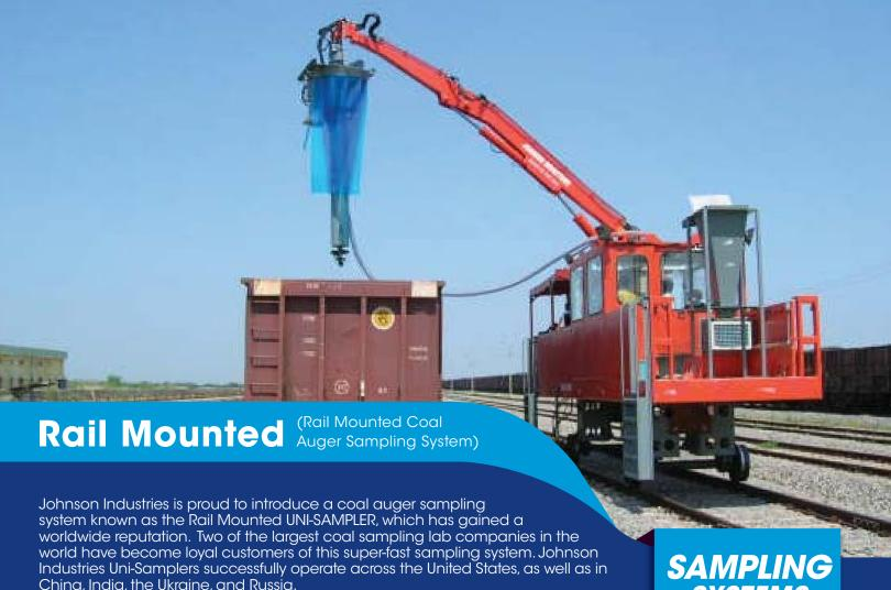
As with any commodity, the coal consumer and supplier want to be assured they are receiving and supplying the correct quality of product. The Uni-Sampler was developed to retrieve coal samples for testing from coal trucks, rail cars, and river or ocean barges. Depending on the customer need, the Uni-Sampler can be manufactured as a stationary pier-mounted unit, a mobile unit, a rail-mounted unit, or a boat/barge mounted unit.
