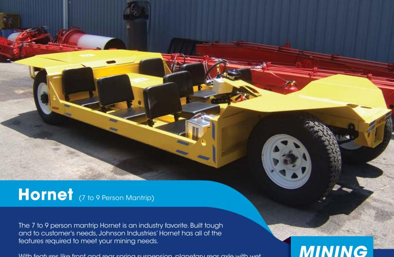
With features like front and rear spring suspension, planetary rear axle with wet brakes, and a 9HP, 48 Volt traction motor with gearbox reducer, the Hornet is a great benefit in a variety of industries. Johnson Industries' 7 to 9 person Hornet has the durability for the job, and is the perfect personnel carrier for salt mines, coal mines, molybdenum mines, zinc mines, potash mines, gold mines, rock mines.
