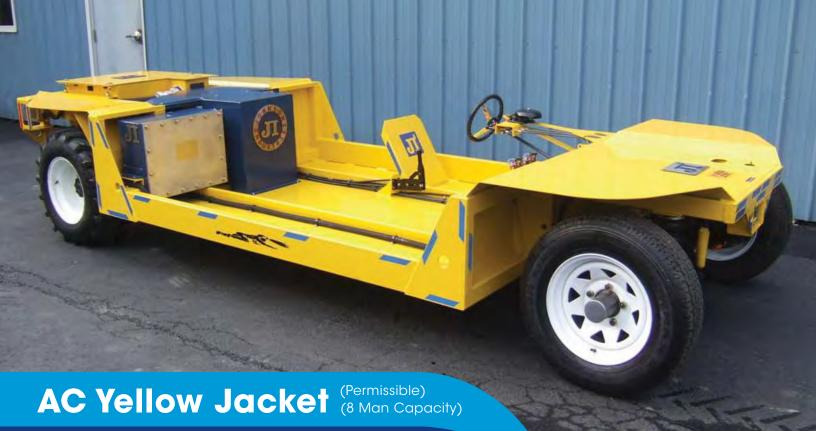
Designed and built for ruggedness and permissibility, the Yellow Jacket is generally used to carry up to 8 workers to the working face of a mine, but it can be used safely in any environment with explosive gas/air mixtures. The AC Yellow Jacket takes this to the next level with more run time and more power. The Yellow Jacket can be equipped with seats for comfort, if the overall height of the mine permits.
