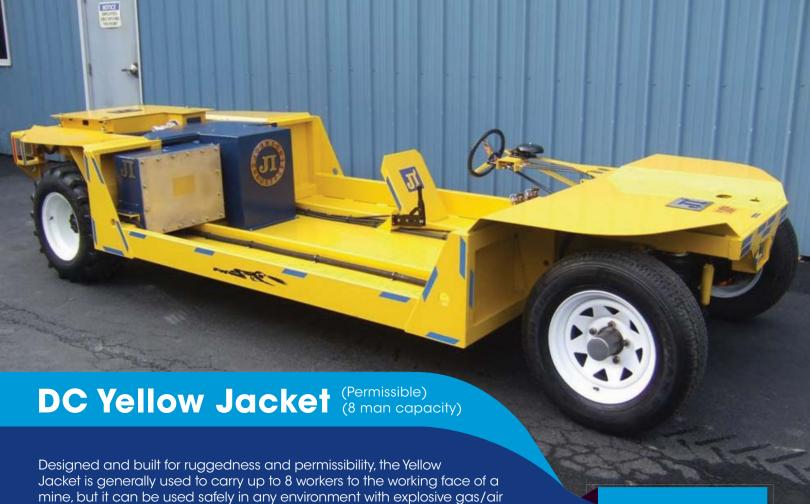
mixtures. The Yellow Jacket can be equipped with seats for comfort, if the overall height of the mine permits.
